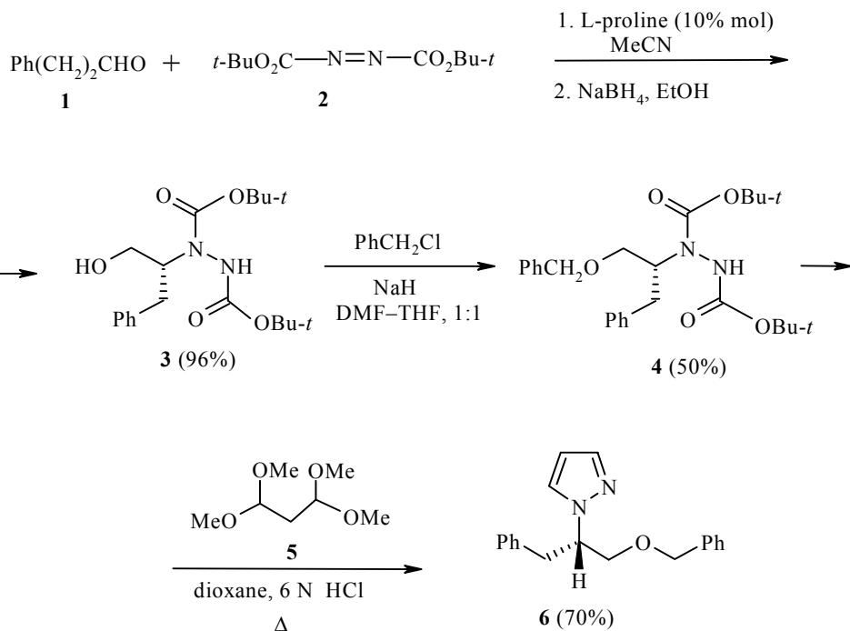
For example, interaction of di-*tert*-butyl azadicarboxylate (2), catalyzed by L-proline, with 3-phenylpropanal (1) at 0°C in acetonitrile with subsequent reduction with NaBH<sub>4</sub> *in situ* led to the formation of di-*tert*-butyl 1-[1-benzyl-2-hydroxy)ethyl]hydrazine-1,2-dicarboxylate (3). Reduction of the aldehyde group is necessary to prevent racemization in subsequent cyclization to pyrazole in acid medium.
